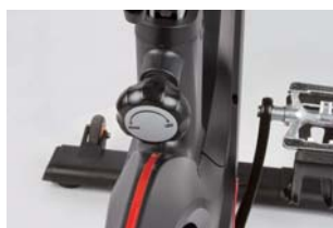
Seat and handlebar height adjustments have locking pop pin for increased safety
